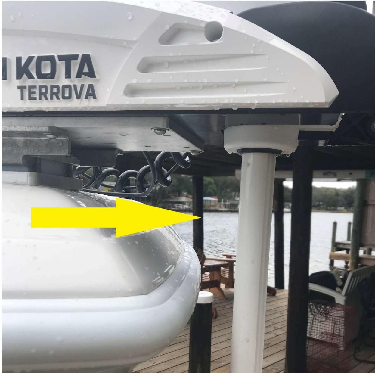
This picture shows how the BMAP-RE is attached directly to a trolling motor without using an additional quick release mount.
